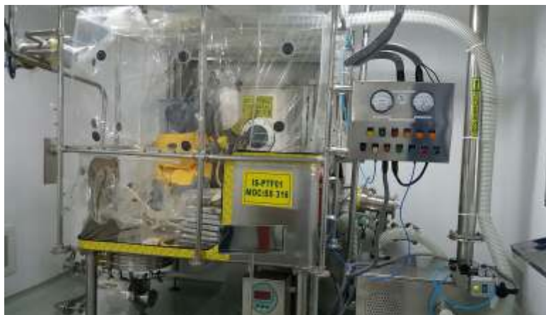
Above: Operator 1/2 Suit Barrier Isolator (internal working) where the dryer equipment is fully enclosed
