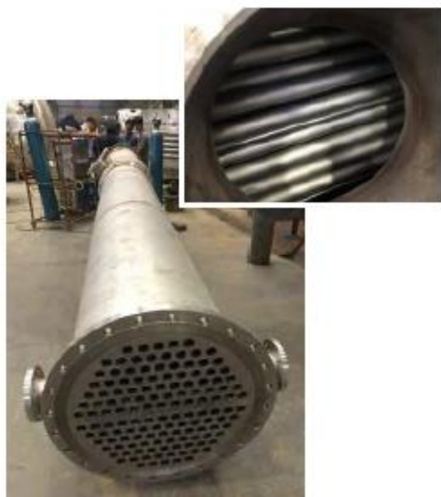
S2 Customised Heat Exchanger: Exotic Alloy (T2) Materials x 4m long
